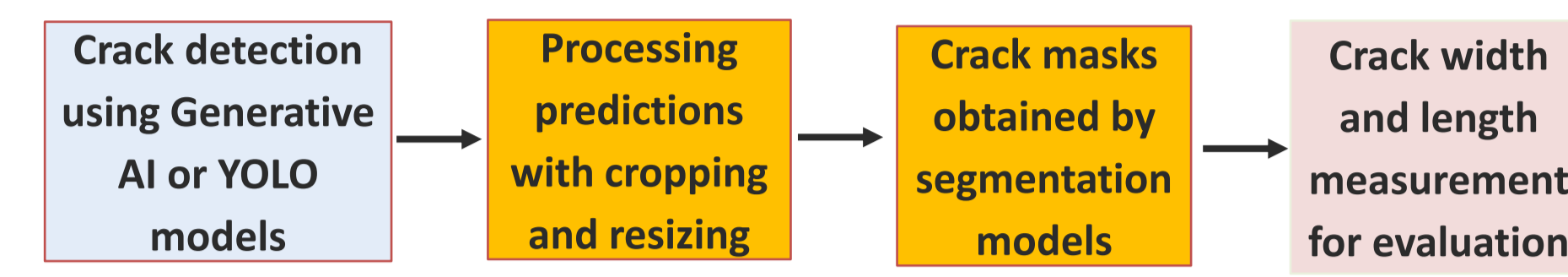
Figure 3 Flowchart of using crack detection and measurement models for pavement crack quantification.
