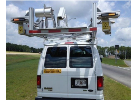
Georgia Tech Sensing Van with an installed 3D laser imaging system
