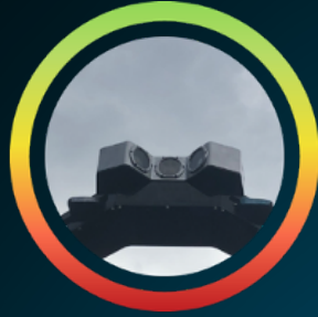
Right of Way cameras deliver 360° imagery
