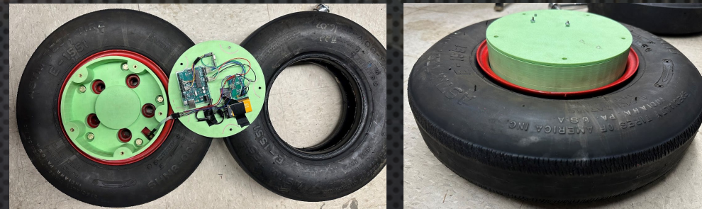
Tire assembly with the new instrument plate attached
