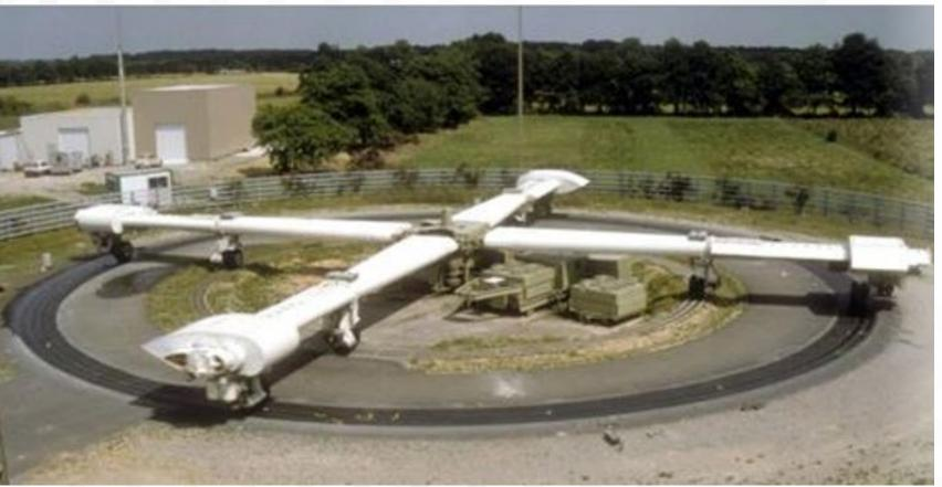
(APT) accelerated pavement testing
