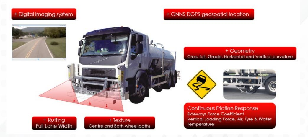
Friction + Geometry + Rutting + Texture + Imaging + Location
