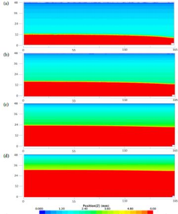
Figure 5-13: Water surface on a 4 lane roadway with a curb and drainage, with 1% cross slope, no longitudinal slope, and at rain intensity (a) 2 in/hr, (b) 5 in/hr, (c) 10 in/hr, and (d) 20 in/hr (curb overflow). The length scale of the computational domain is in feet.
