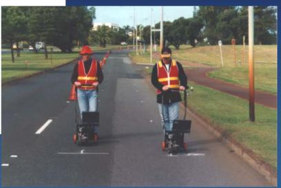
Verification of IRI measurement via comparison with Class 1 profile measuring device e.g. Walking Profiler
