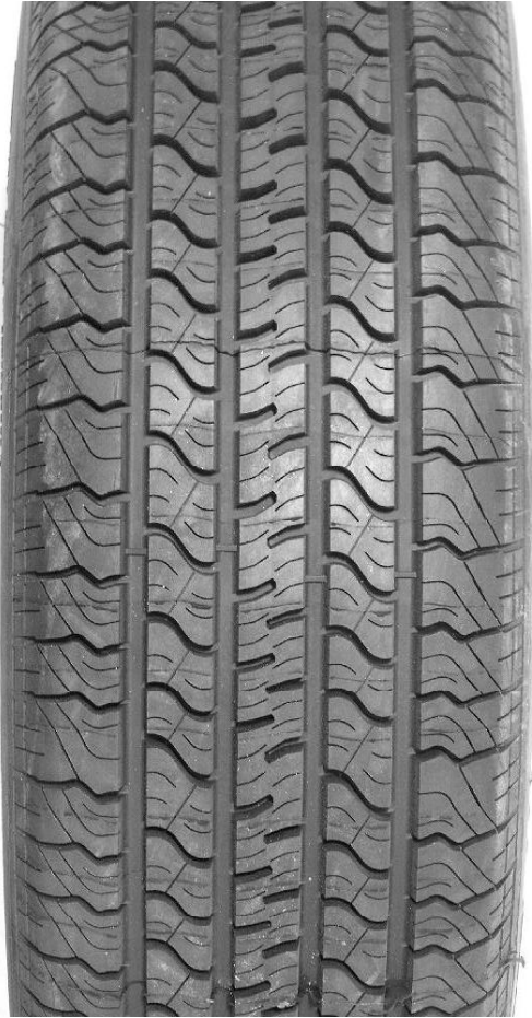
ASTM F 2493 Standard Reference Test Tire (SRTT)
