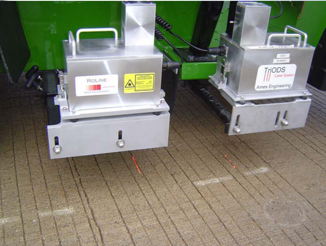
RoLine and TriODS sensors mounted on lightweight profiler.
