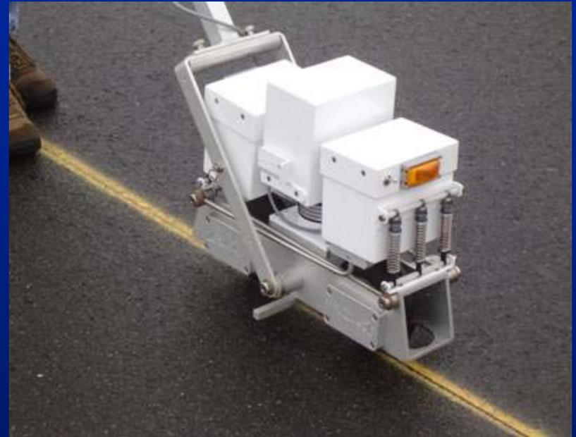
**Able to obtain data at 1-inch interval at walking speeds**
