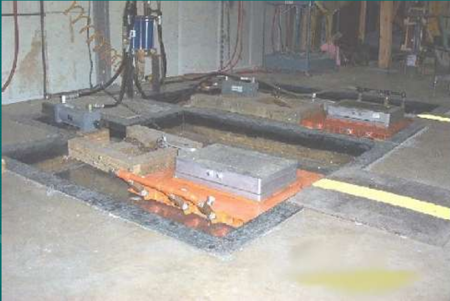
Fig. 2(a) In-House Transducer Calibration Platform
