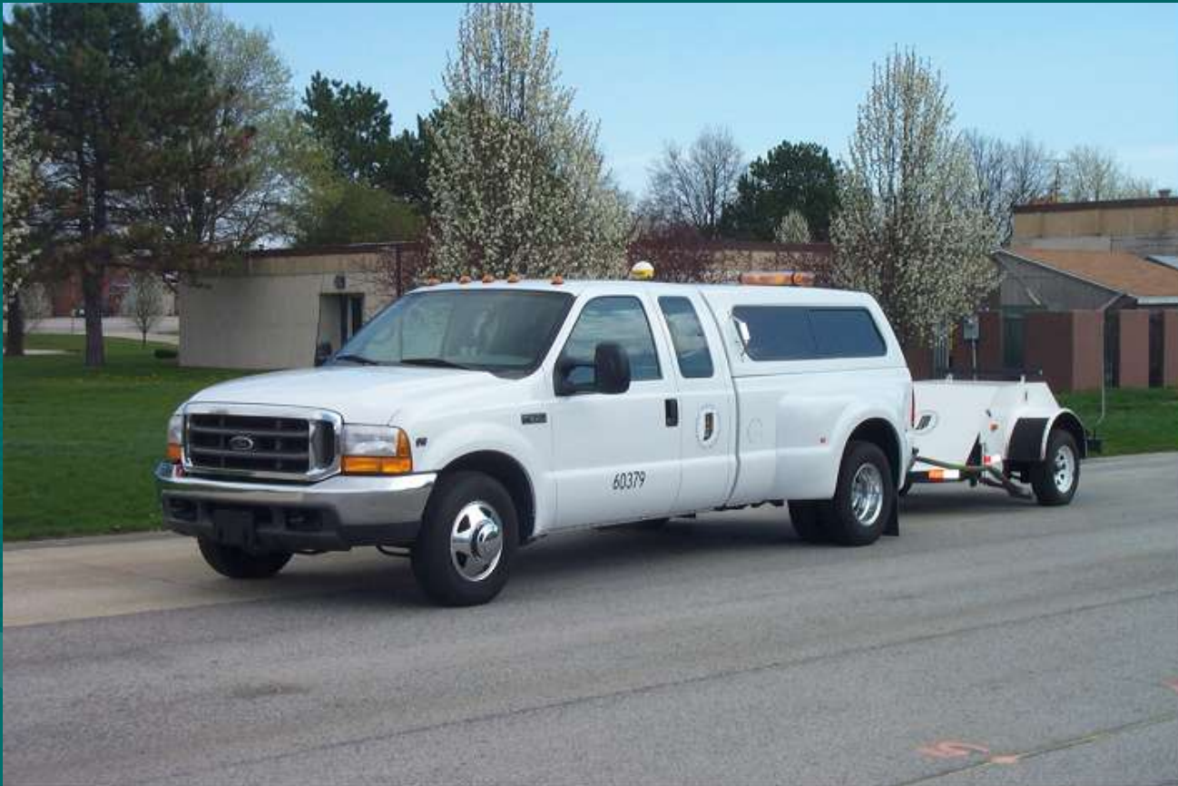
Fig. 1 ASTM E-274 Locked-Wheel Tester
